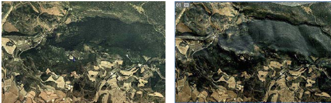
Fig. 3. Left: An original orthoimage of Navarre, Spain (Northern Hemisphere). Right: the same image but transformed using a superimposed artificial hill shading model with 315° azimuth and 45° altitude for a top-left lighting.
