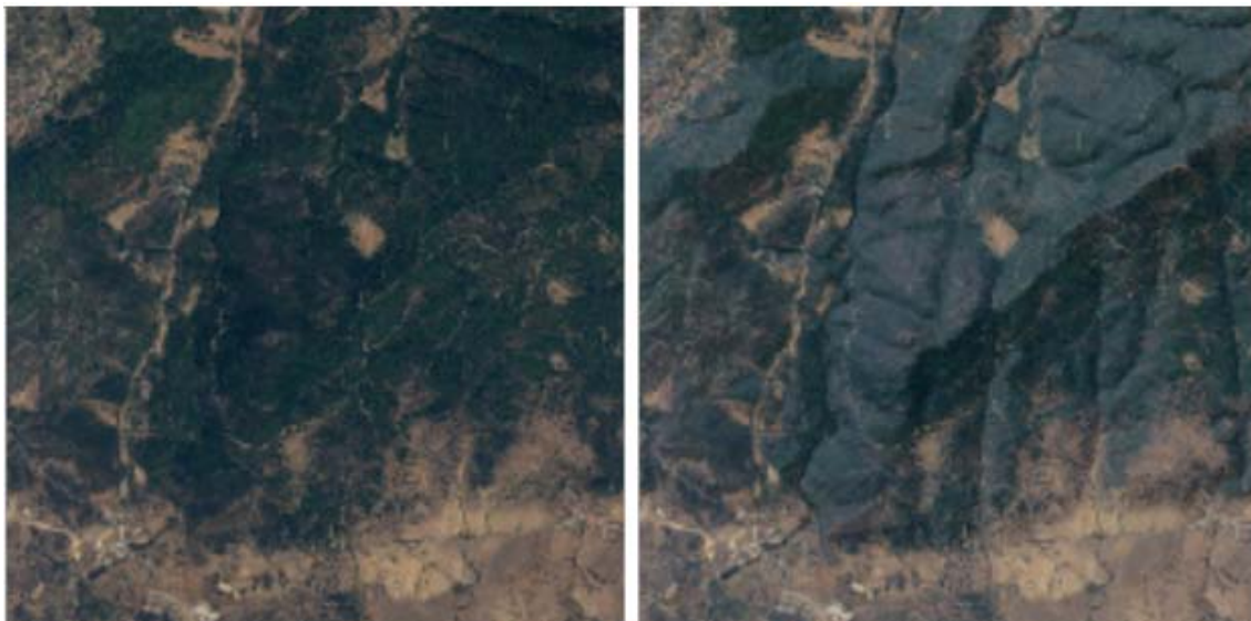
Fig. 6. Close-up of original (left) and processed (right) orthophoto with overlaid semitransparent hill shading model. Original image courtesy of the Instituto de Tecnologías Agrarias de Castilla y León.
