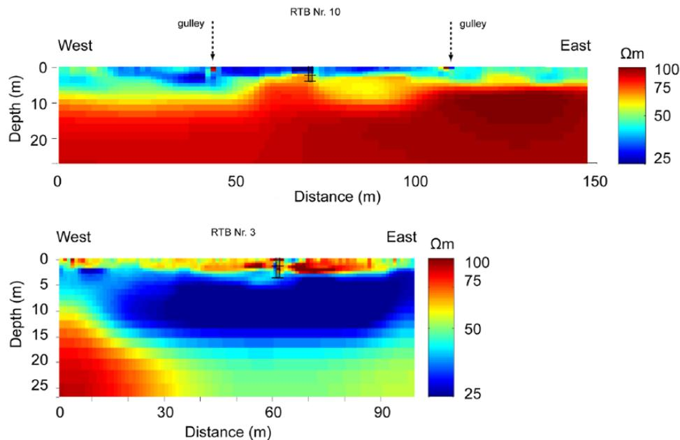
**Figure 5.** Tomograms (electrical resistivity of the subsurface given in  $\Omega\text{m}$ ) of site 10 (above) and 3 (below). Electrode spacing at site 10 was 1.5 m and at site 3, 1 m.
