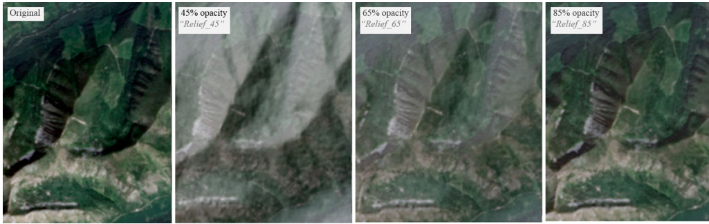
Figure 2. An illustration of how the changing opacity levels affect the outcome with the SRM overlay solution. Left to right: original satellite image, SRM overlain with 45%, 65%, and 85% opacity levels.
