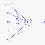
Every unit in an ANN performs a simple operation: apply a activation function, f(), to weighted sum of its inputs.
